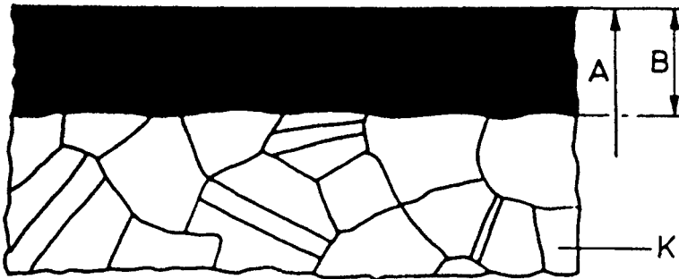
Fig. 3-28: Uniform material disintegration corrosion shown schematically A Starting condition B Material thickness disintegration of the part due to uniform corrosion K Grain (crystal)
