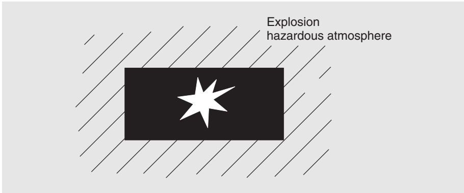
Fig. 7-4: Potted encapsulation schematic
