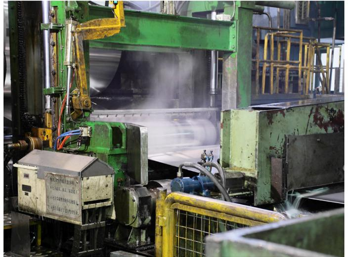
Last pass - Stressometer roll in measuring position
