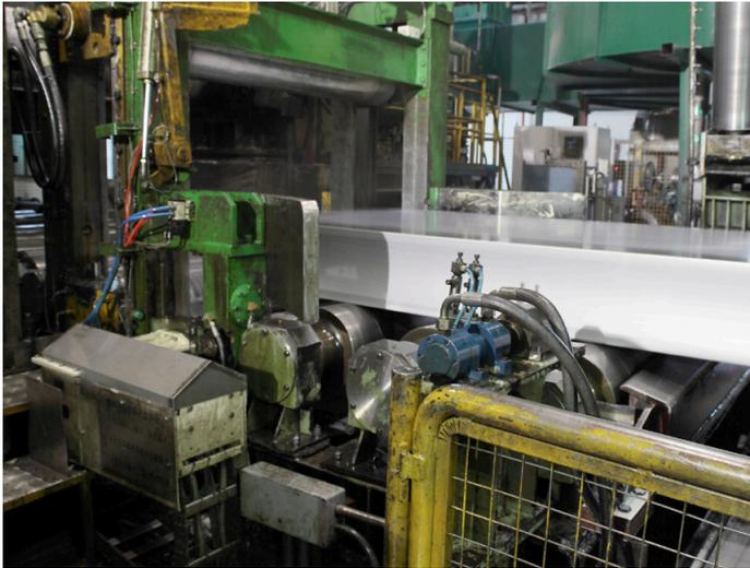
First pass - Stressometer roll in lower position
