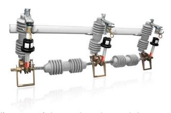
If a permanent fault occurs, the continuous reclosing operations do not clear the fault. However, the three-phase AutoLink counts these operations and, when one or more AutoLinks reach the set count, the AutoLink opens the three-phase network.
