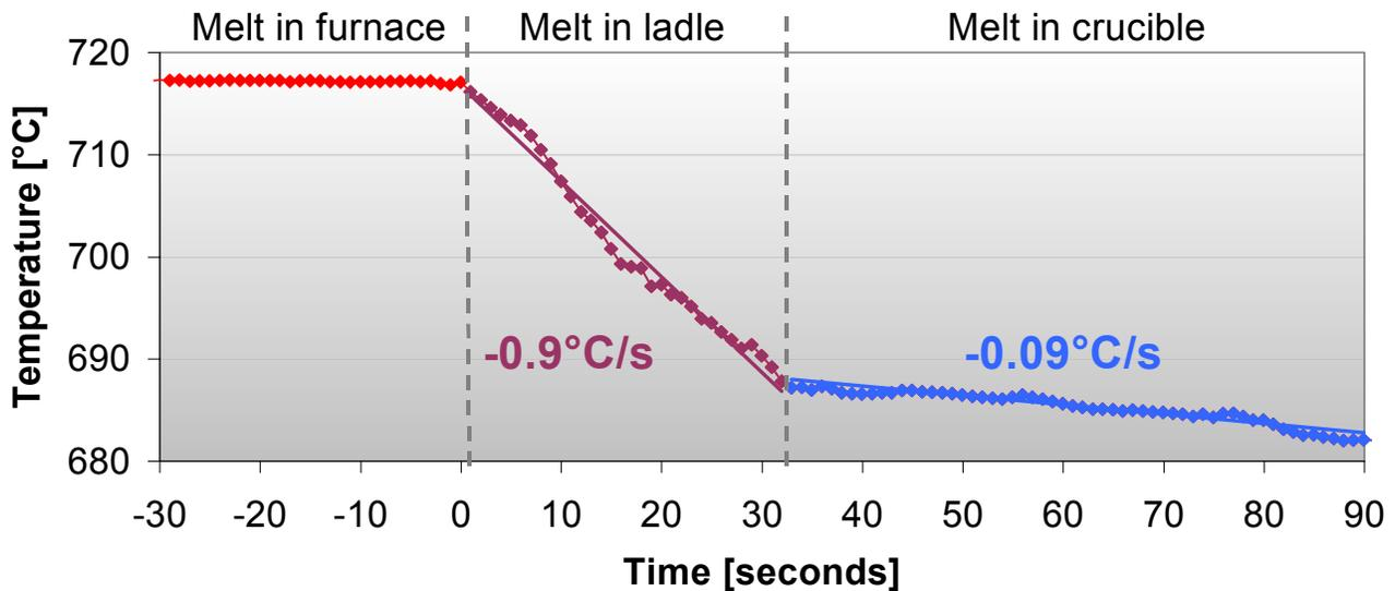
Figure 1: The most significant heat loss occurs when the metal is in the ladle (see PoDFA Eng Bulletin No. 1)
