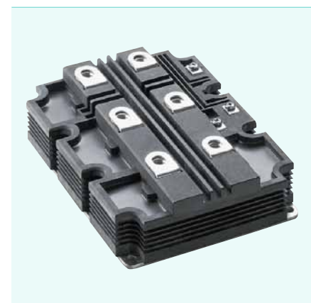
5 The 6.5 kV HV-HiPak module comprising the newly developed SPT+ chip-set
