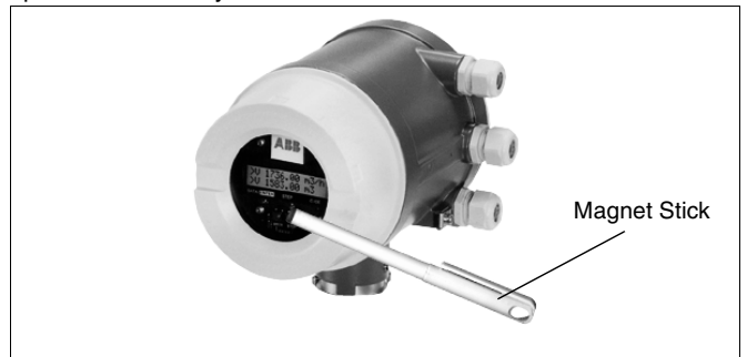
Fig. 15 Magnet Stick Operation
