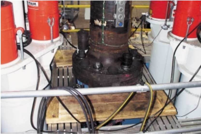
2 HMF riser flange being tension-tested (API class F rating to 2500 kips tension)
