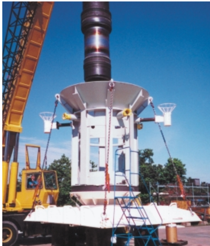
5 Super MS-700 subsea wellhead and guidelineless re-entry assembly (GRA)
