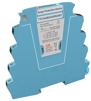
Combined Category D, C, B tested protector (to BS EN 61643) suitable for twisted pair signalling applications within hazardous environments (ATEX/IECEx approved). Available for working voltages of up to 15 and 30 Volts. For use at boundaries up to LPZ 0 to protect against flashover through to LPZ 3 to protect sensitive electronic equipment.
