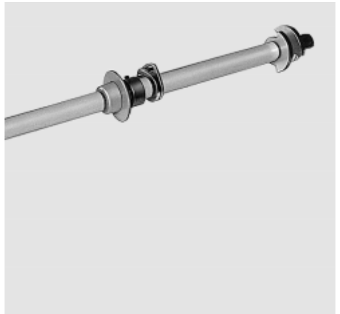
Figure 5/24: The earthing switch drive shaft is supplied loose when the top mounted enclosures are removed for transport purposes. View for the open position of the earthing switch with individual mechanism parts fitted in the positions for correct function.
