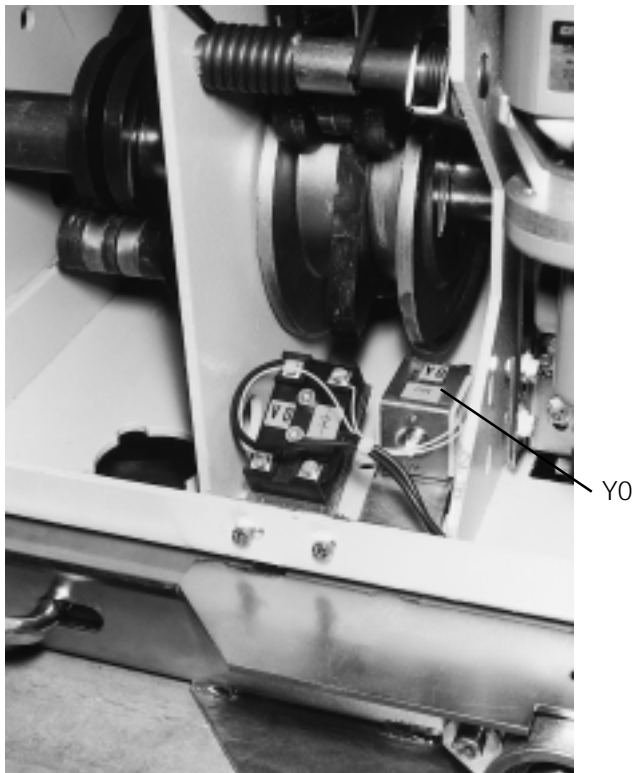
Figure 7/7: Manually moveable withdrawable part, front panel removed.
