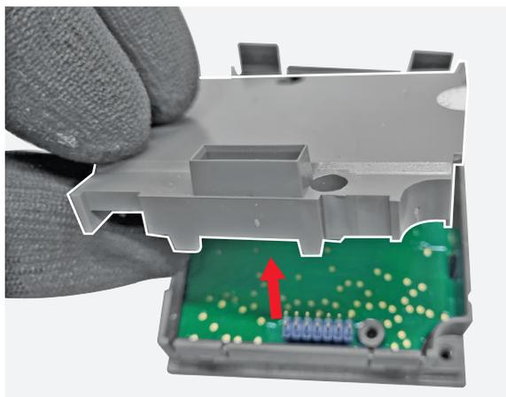
**38** Manually remove the printed circuit board.
