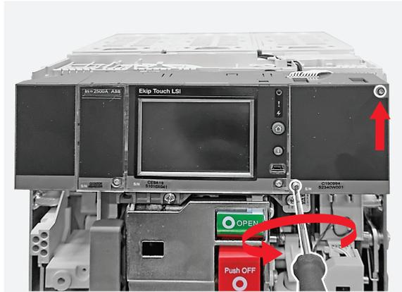
**34** By means of the flat screwdriver unhook the Ekip measuring blind module from the trip unit and after manually complete the removal.
