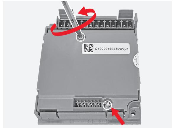
**37** Manually remove the Ekip measuring blind case.
