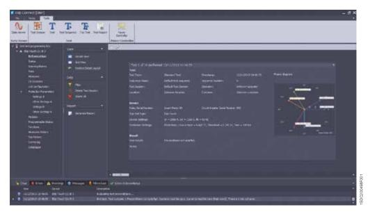
Ekip Connect automatically scans the RS-485 bus, detects all the devices connected and checks their configuration, checking all the possible address, parity and baud rate combinations. A simple click over SCAN will highlight:
