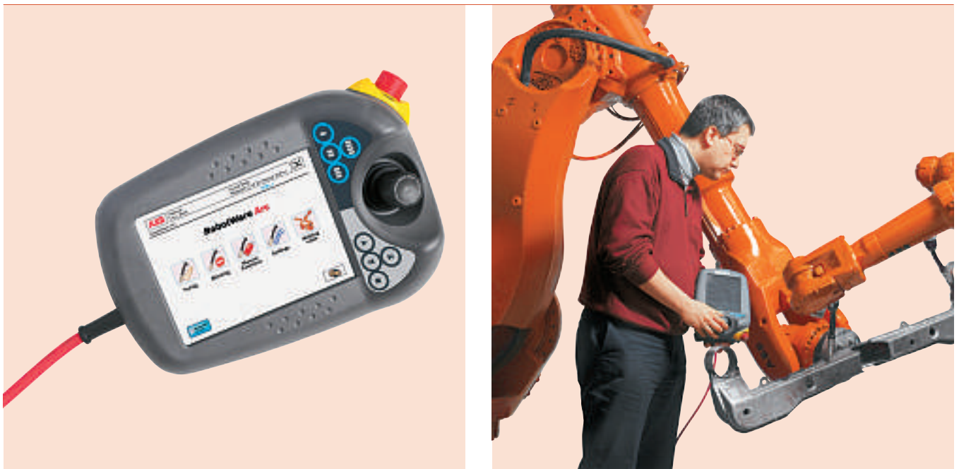
2 ABB's Flexpendant (a) is part of the IRC5 package. It supports robot programmers (b) through its ergonomic design, customized menus and touch screen.
