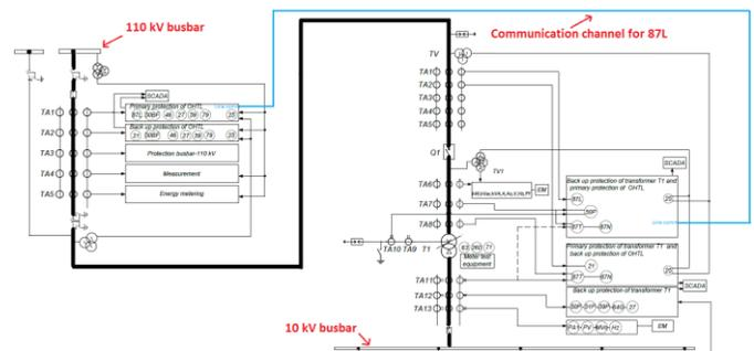
Fig. 2 – SLD diagram showing the 110/10 kV step-up transformer connecting the solar power-plant to the 110 kV system
