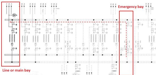
Fig. 1 - SLD of the station where the line can be supplied from the main bay, with the CT ratio 500/5 A, or from the emergency bay, with the CT ratio 600/5 A. Due to different CT ratios for the protected object, this represents a challenge for most protection IEDs
