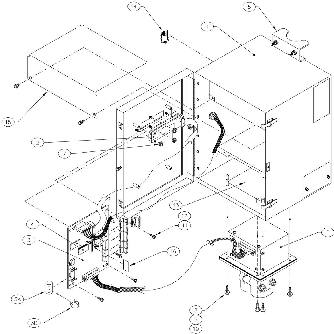
**Figure 5-2 6413 FCU Component/Cable Locations**
