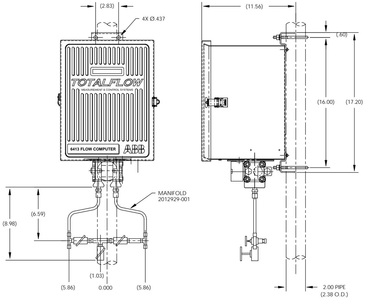
**Figure 2-5. Model 6413, Pipe Mounting W/Discrete Manifold**
