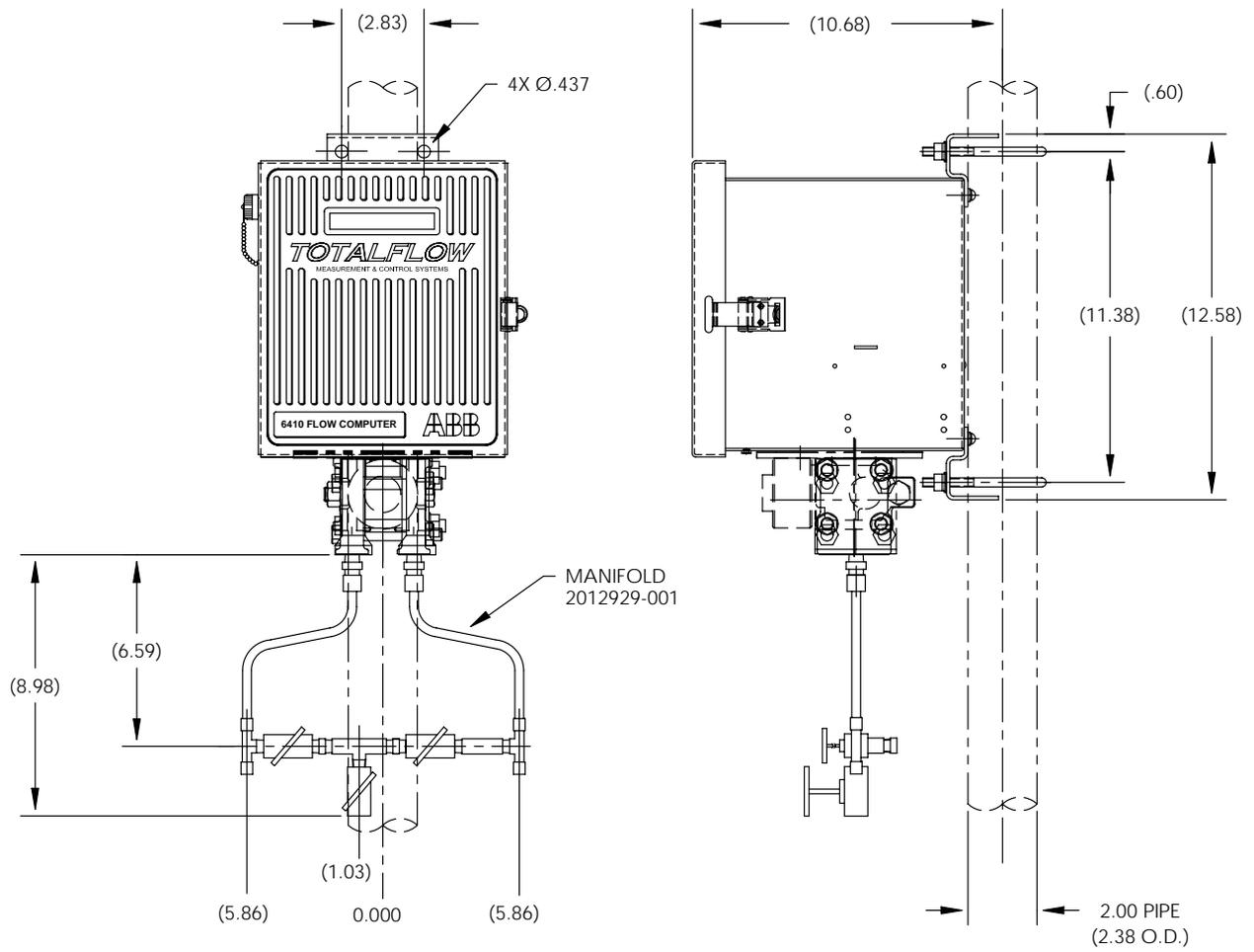
**Figure 2-4. Model 6410, Pipe Mounting W/Discrete Manifold**
