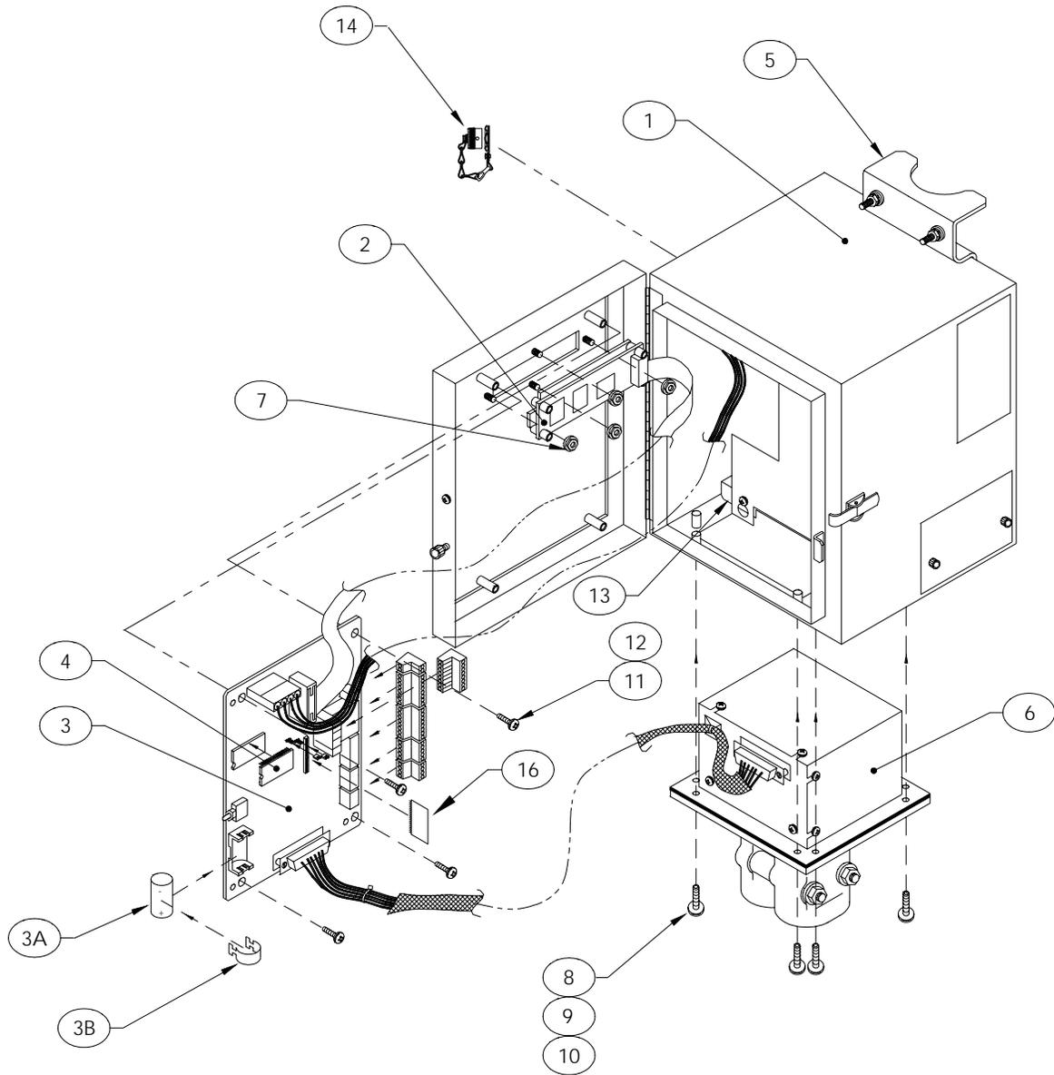
**Figure 5-1 6410 FCU Component/Cable Locations**
