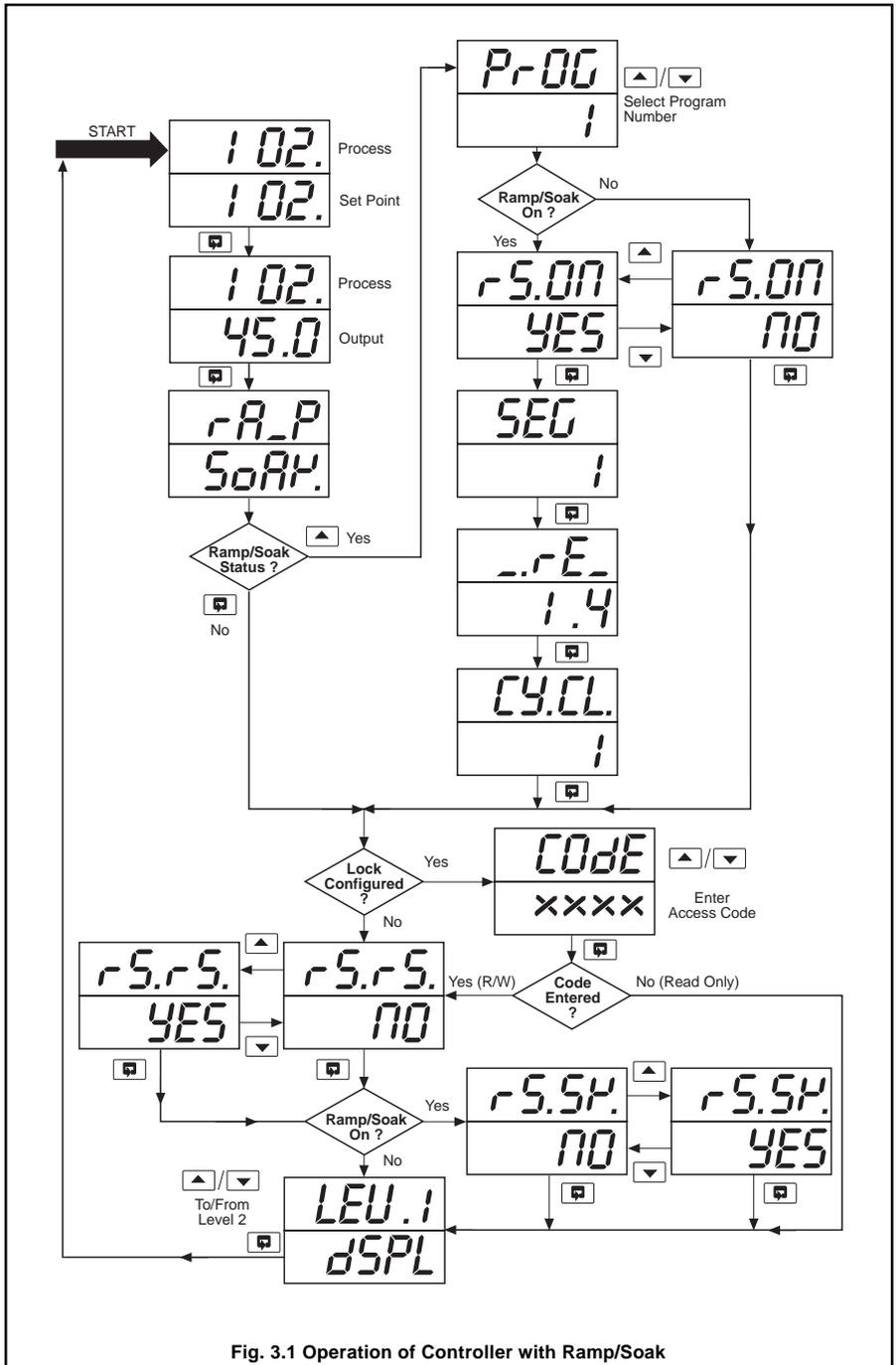
Fig. 3.1 Operation of Controller with Ramp/Soak
