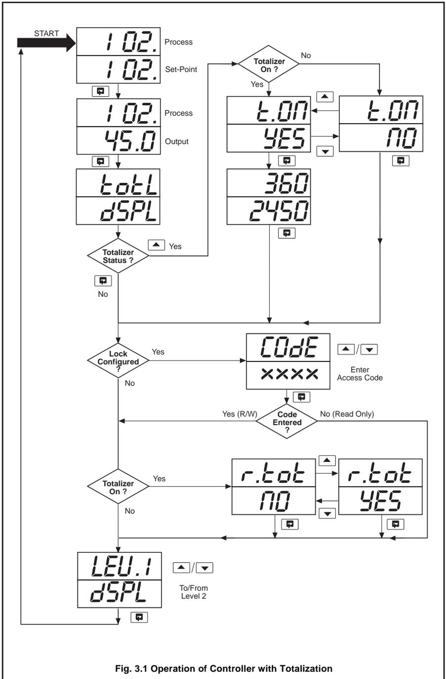
Fig. 3.1 Operation of Controller with Totalization
