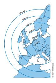
The D 365 DCF77 antenna receives scheduled messages broadcasted from the DCF77 emitter located in Mainflingen, Germany. The broadcast power is 50kW with a range of 2500 km. Sometimes the signal is received intermittently and not all locations may be covered due to shadows caused by the land, especially in countries far away from the emitter; in any case, Italy has full coverage.
