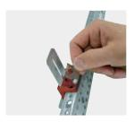
To enable double insulated mounting, simply remove the metal plate from the deep-mounting bracket. Once you have done this, no other insulation parts are required. Mounting and stepless depth adjustment can be carried out from the front, for optimum handling.
