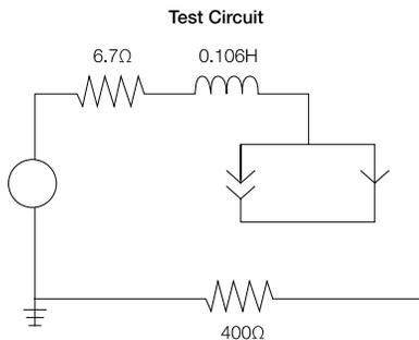
The applied voltage was selected at 27.5kV, much in excess of normal line-to-ground voltage, to increase the failure rate. This allowed evaluation of test and design parameters with a limited number of samples.
