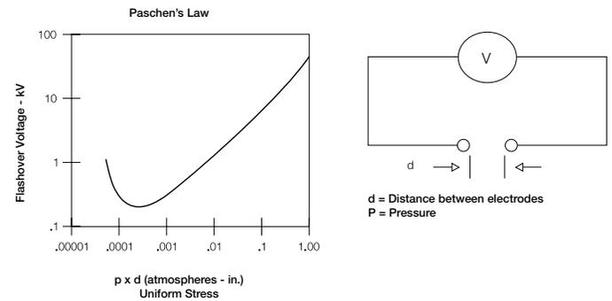
To see the effect of pressure, let  $d = 1$  inch. The horizontal axis then represents pressure only. Note that at 1.0 atmosphere, the flashover voltage for 1 inch is approximately 60kV, and at 0.1 atmosphere, the flashover voltage decreases to approximately 8kV.
