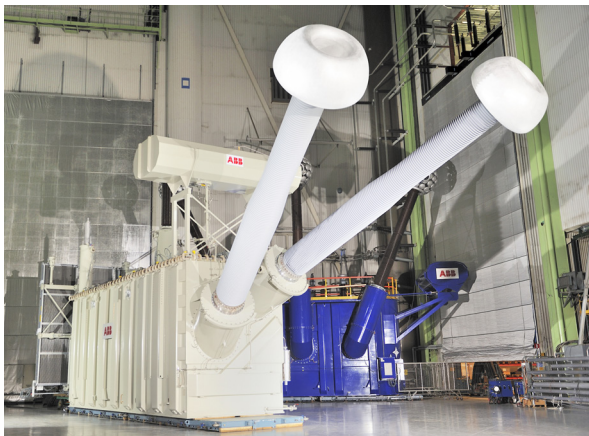
ABB's 800 kV ultrahigh-voltage DC transformer - a key component for long-distance, bulk power transmission systems - will be used in world's longest power transmission link in China
