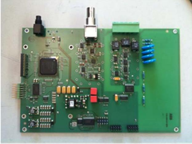
**Figure 3 Active detector unit with high speed A/D conversion and wave shape memory**
