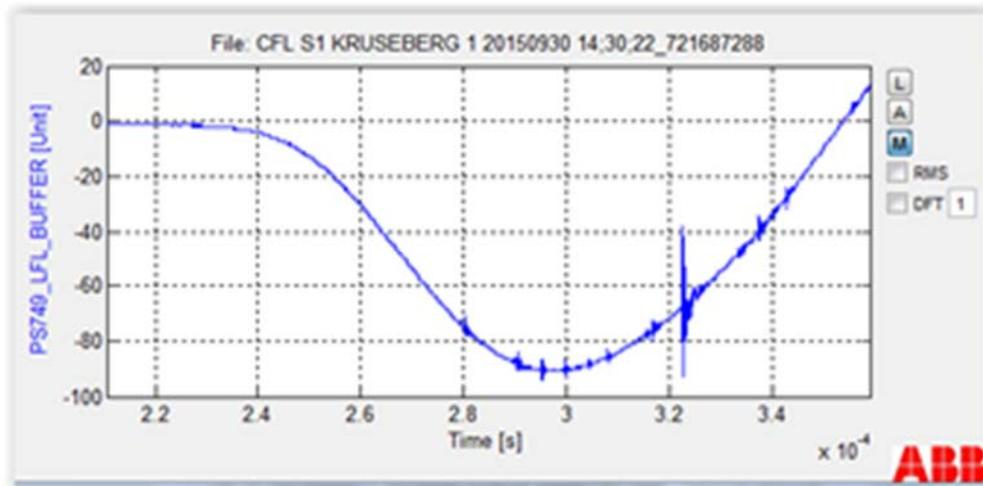
Figure 7 Staged fault in Herrenwyk, transient recorded in Kruseberg
