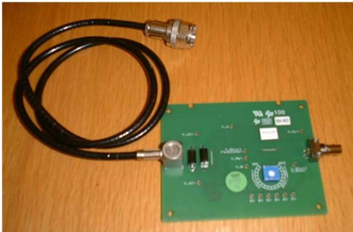
**Figure 2 Passive detector unit with optical output**
