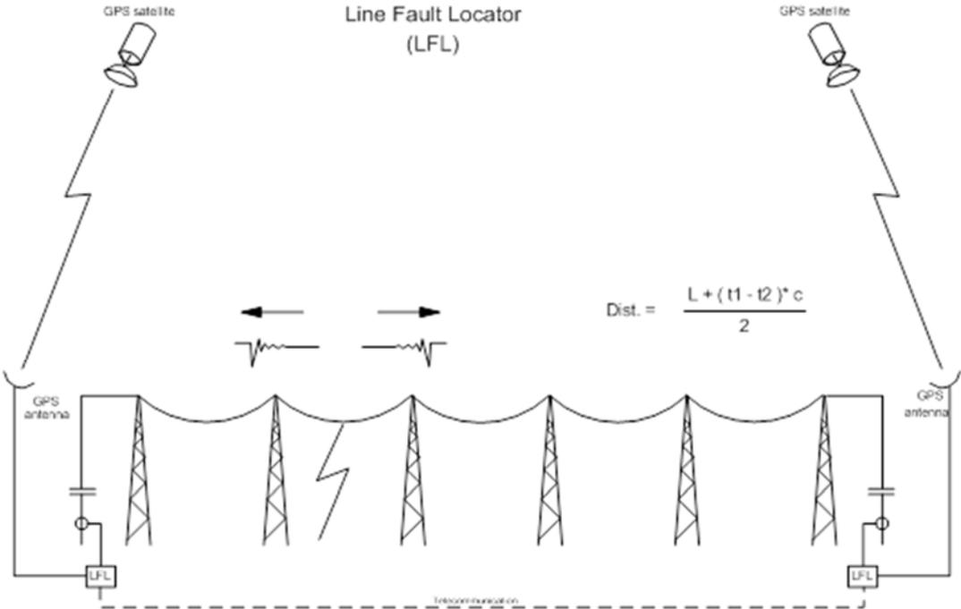
**Figure 1 Principle of the two sided Line Fault Locator with GPS clock synchronization**
