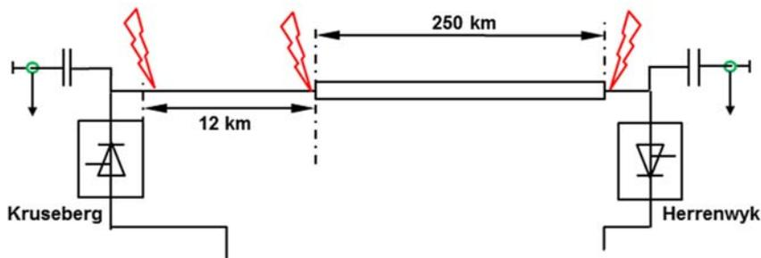
**Figure 5** Simplified view of Baltic Cable to indicate staged fault locations for Cable Fault Locator testing
