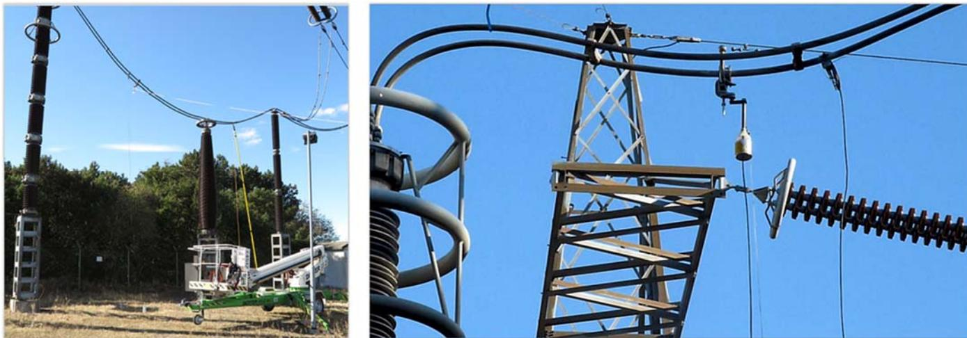
**Figure 6** Staged fault device used for OFL tests in Baltic Cable
