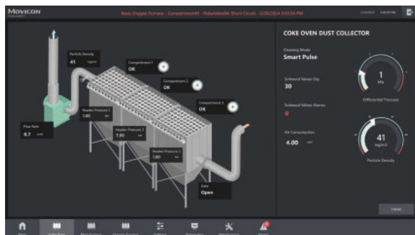
▲ Emerson’s Movicon.NEXT HMI/SCADA software platform goes beyond just providing basic visualization of a coke oven dust collector (shown). It also supports IIoT integration, offers local and remote user-interface options, supports cybersecure connectivity, and works with on-premises, hybrid, and cloud-based architectures. Source: Emerson
