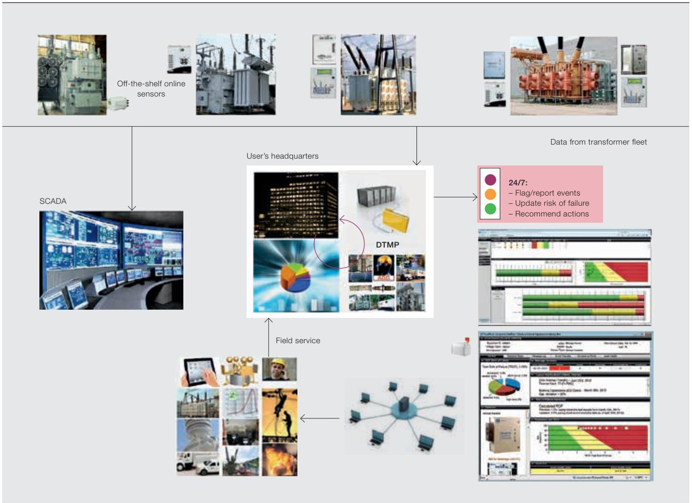
An expert system algorithm is then able to look at a transformer as a whole instead of at its individual components, as a health index would.
