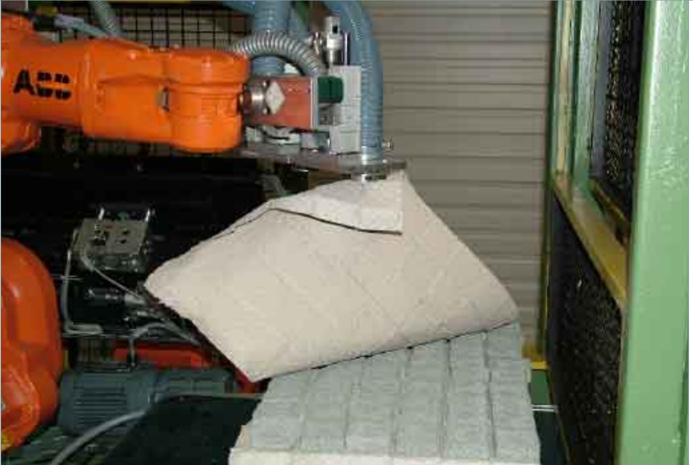
An IRB 140 robot picks up a filter from the stack.
