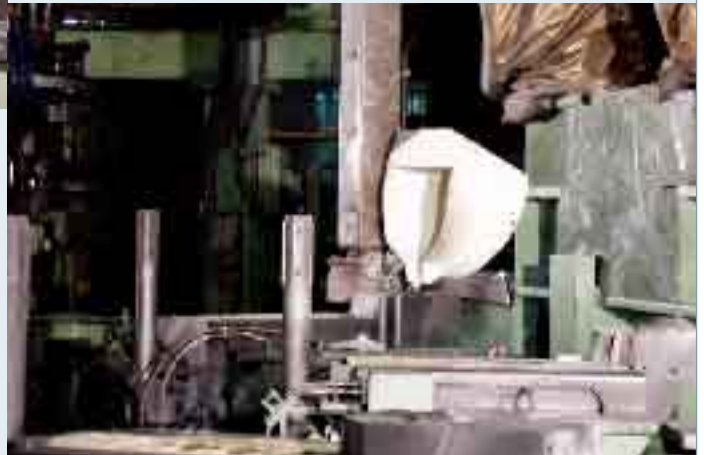
Two robots take turns loading and pouring aluminum.
