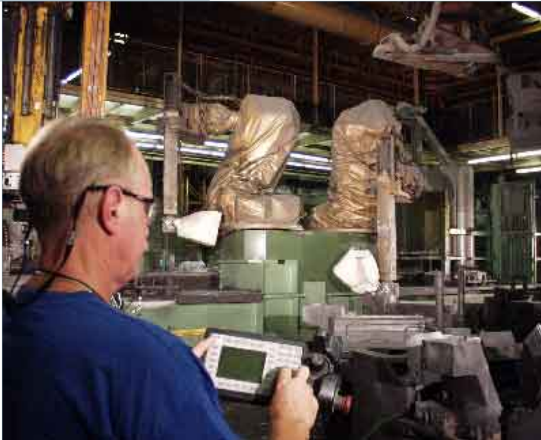
Monitoring the robot is easy with the Flex-Pendant.
