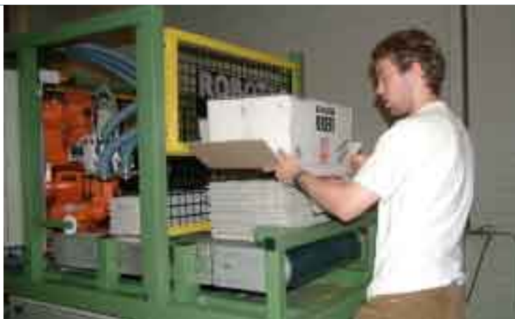
Placing filters on the conveyer is the only manual part of the operation.
