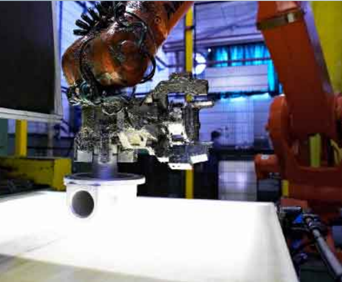
A robot deposits a lubricated filter on a slide.
