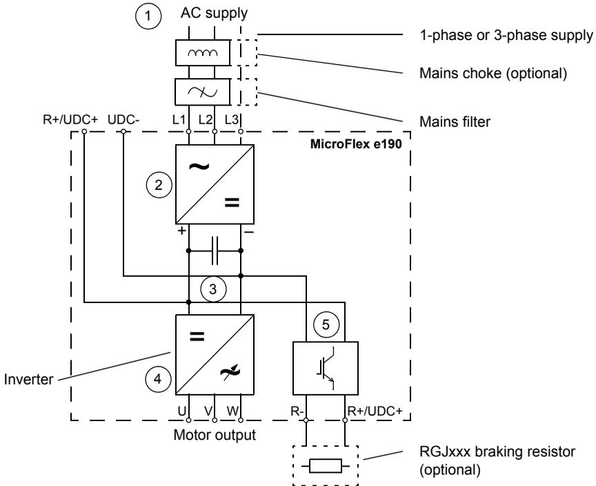
1. AC supply. 1-phase 200...240 V or 3-phase 200...240 V phase-to-phase ( $\pm 10\%$ ).
