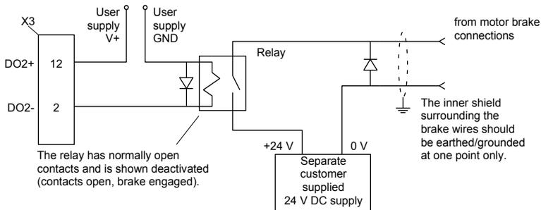
This circuit uses DO2 as a motor brake output. The output is configured using Mint keyword `MOTORBRAKEOUTPUT`; see the Mint help file for details. With this configuration, the following sequences can be used to control the brake.
