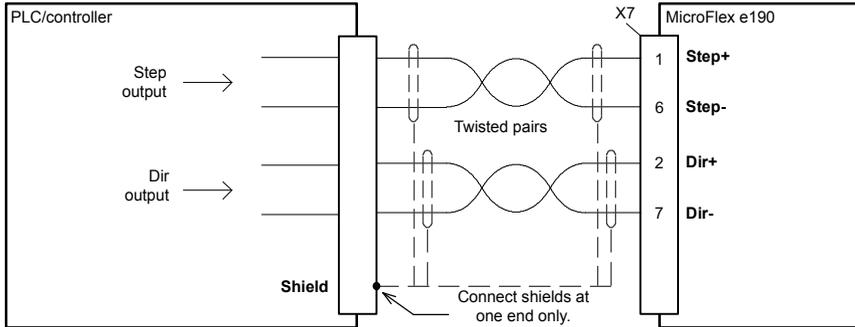
**Note:** The inputs should be use shielded twisted pair cable with an overall shield. Connect the input signals correctly according to the pin assignment for connector X7.
