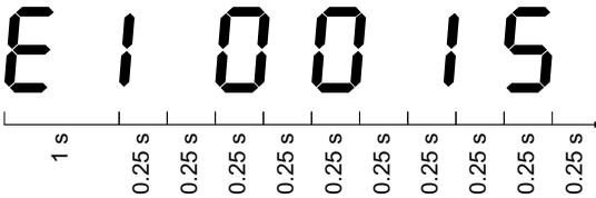
The decimal point to the right of the number also illuminates to indicate STO errors. If a **b** symbol appears followed by an error code, please contact ABB technical support. For a complete list of error codes, open Mint WorkBench, press F1, and locate the Error Handling book. This contains topics listing the drive status display indicators and basic error codes. See also [Start the MicroFlex e190](#) on page 95.
