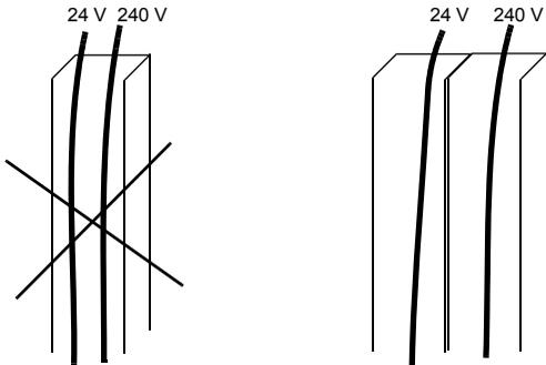
Not allowed unless the 24 V cable is insulated for 240 V or insulated with an insulation sleeving for 240 V.
