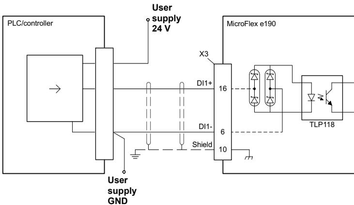
Digital input - typical connections from an ABB DO561 PLC output module:
