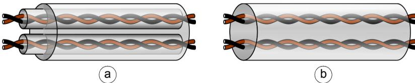
Run analog and digital signals in separate cables.
