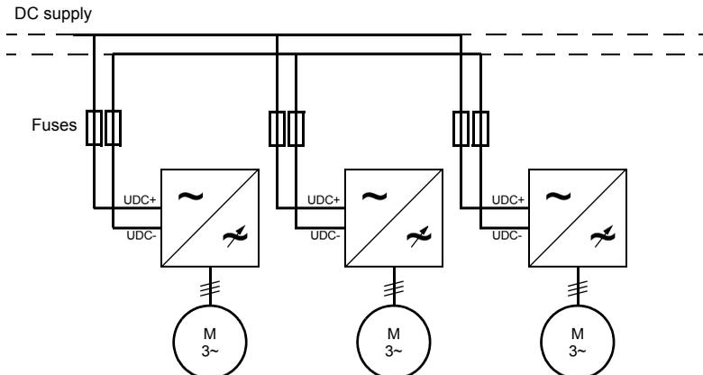
Each drive has an independent DC capacitor pre-charging circuit.
