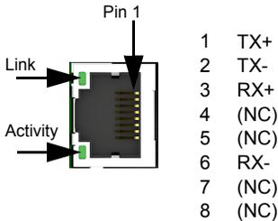
The E1 and E2 Ethernet ports on the top panel of the MicroFlex e190 are used for real-time Ethernet fieldbus connections such as EtherCAT® and Ethernet POWERLINK®. For full details about the fieldbus connections, see the Mint WorkBench help file.
