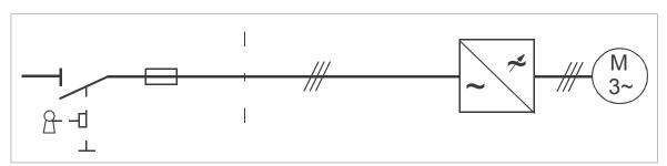
Select the fuses or circuit breakers according to local regulations for the input cable protection. Select the fuses or circuit breakers for the drive according to the instructions given in the technical data. The fuses or circuit breakers for the drive protection will restrict drive damage and prevent damage to adjoining equipment in case of a short-circuit inside the drive.
