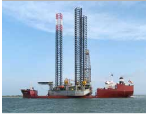
8 A semisubmersible heavy lift vessel with rig on deck and OCTOPUS monitoring and routing system on the bridge
