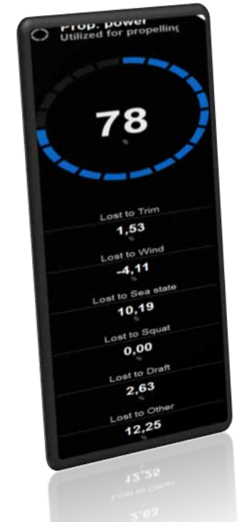
5 Real-time view of the power breakdown seen by the onboard crew. This enables the crew to detect abnormalities and take immediate and timely action.
