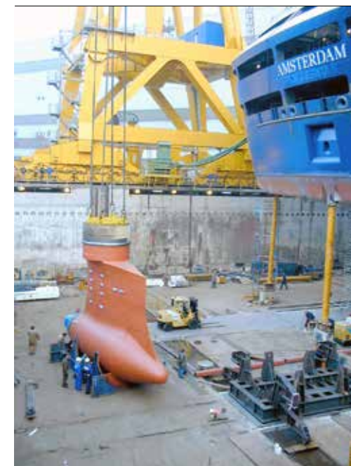
Lloyd’s Register staff oversee the lifting of an Azipod into dock
