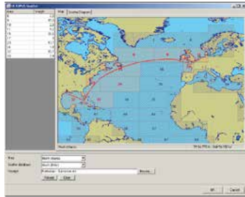
12 Matching of an indicative route plan with a wave scatter diagram database. The passage time per wave area is accounted for.
