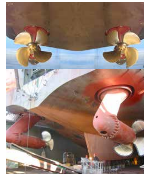
2 Pulling Azipod CO propulsors receive undisturbed water inflow, which increases propeller efficiency.
