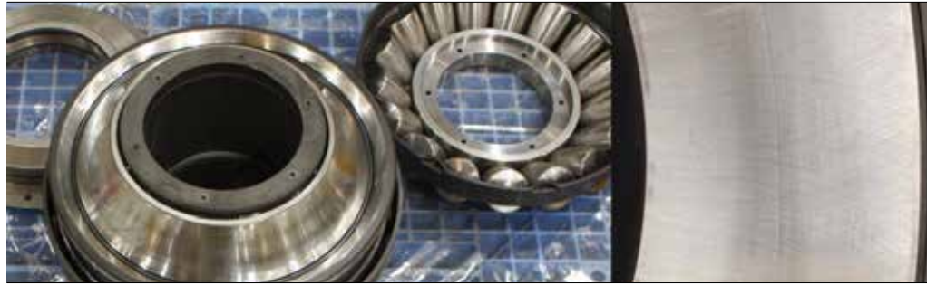
6 Azipod C thrust bearing condition after close to nine years of DP operation. The original grinding texture (right) could still be seen on the raceway.
