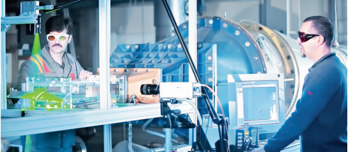
Non-intrusive flow measurement by means of laser optic particle image velocimetry
