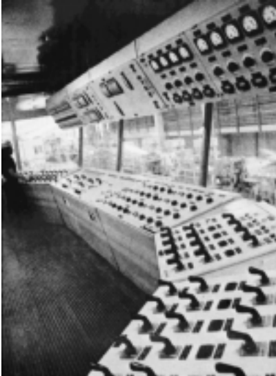
1 Typical control desk in a profile mill. Pushbuttons and potentiometers dominate the scene.
