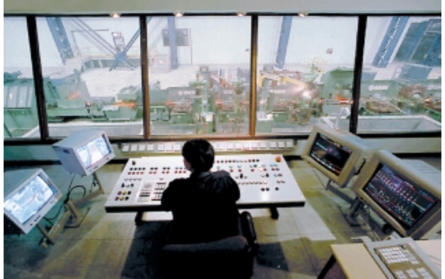
2 State-of-the-art control room. The operator, who works in a Windows environment, supervises the process on-line.
