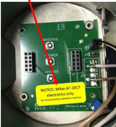
*NOTE: It is important to know that the electronics (M4xx-AT-2017) are not designed to work in the previous generation devices. Additionally, the electronics from the previous generation equipment (M4xxx-AT) will not be functional in the 2017 and later devices.*
