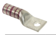
One-hole lugs — long barrel 600 V to 35 kV Material: high-conductivity wrought copper Finish: electro tin plate
