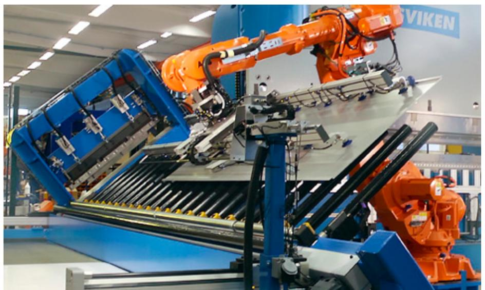
The robot inserts the sheet into the robot controlled press brake tending machine for precise folding.
