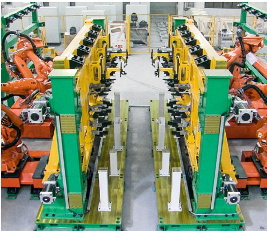
The GateFramer car body system can handle up to six different models on the same line.
