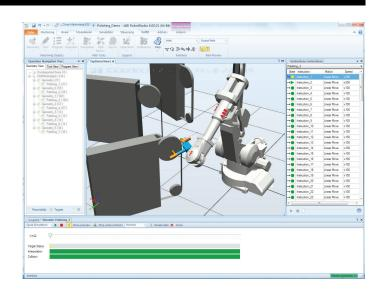
RobotStudio is built on the ABB VirtualController, a replica of the software which runs your robots in production. It allows realistic simulations to be performed, using actual robot programs and configuration files identical to those used on the shop floor.
