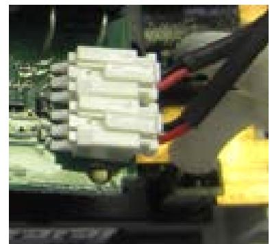
14. Disconnect the fan cable from the sub board.
