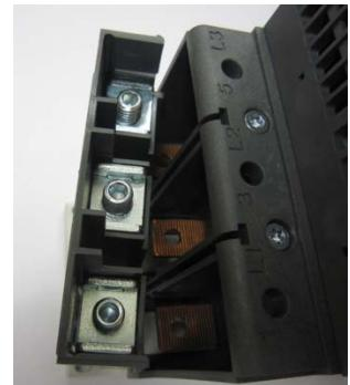
23. Connect the cables to 1L1, 3L2, 5L3 (main voltage) and 2T1, 4T2, 6T3 (motor connection).
