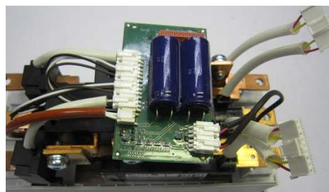
12. Disconnect the sub board from the middle part. Don't remove the cables.
