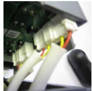
20. For PSE210...370 connect the cable between the main board and the sub board.
