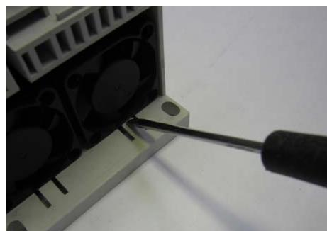
13. Remove the broken fan. The fans are mounted with snaps.
