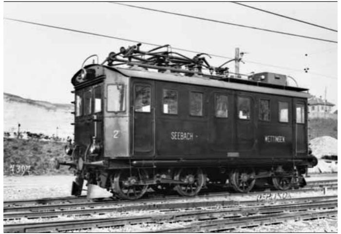
4 MFO experimental locomotive no. 2 with single-phase traction motors
