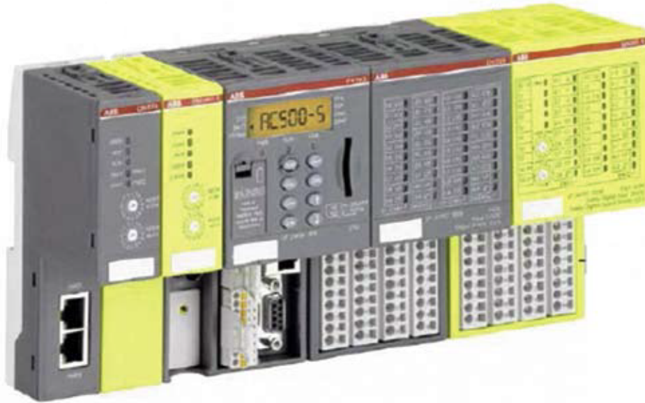
Fig. 3: High speed PLC with five microsecond sampling rate and Industry 4.0 capabilities
