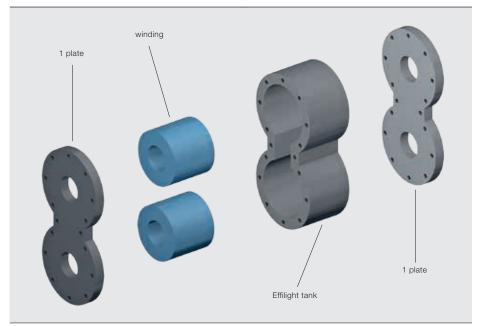
Now that only the windings are immersed in oil, for cooling and dielectric purposes, the oil volume can be reduced by up to 70 percent when compared to a classic transformer.
