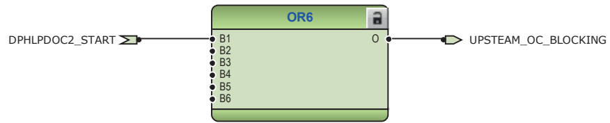
Figure 88: Upstream blocking logic
