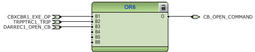
Figure 33: Circuit breaker control logic: Signal for opening of circuit breaker 1
