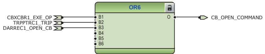
Figure 230: Signals for opening coil of circuit breaker 1
