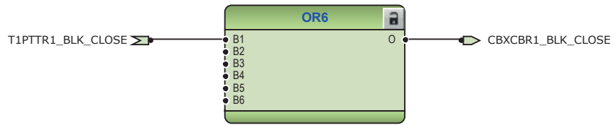
Figure 125: Circuit breaker 1 close blocking logic
