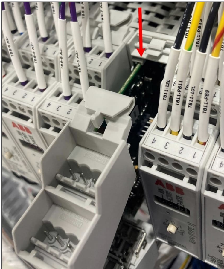
Figure 3-7: Board inserted through the housing guiding rail (top view)
