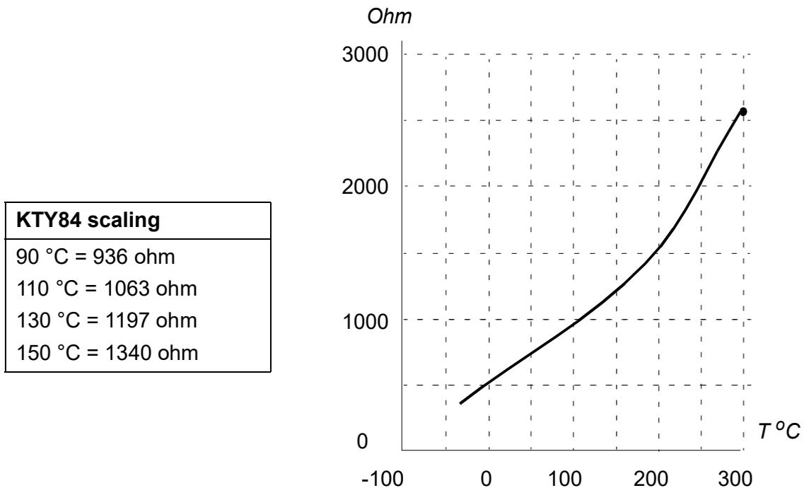
The warning and fault limits can be adjusted by parameters.
