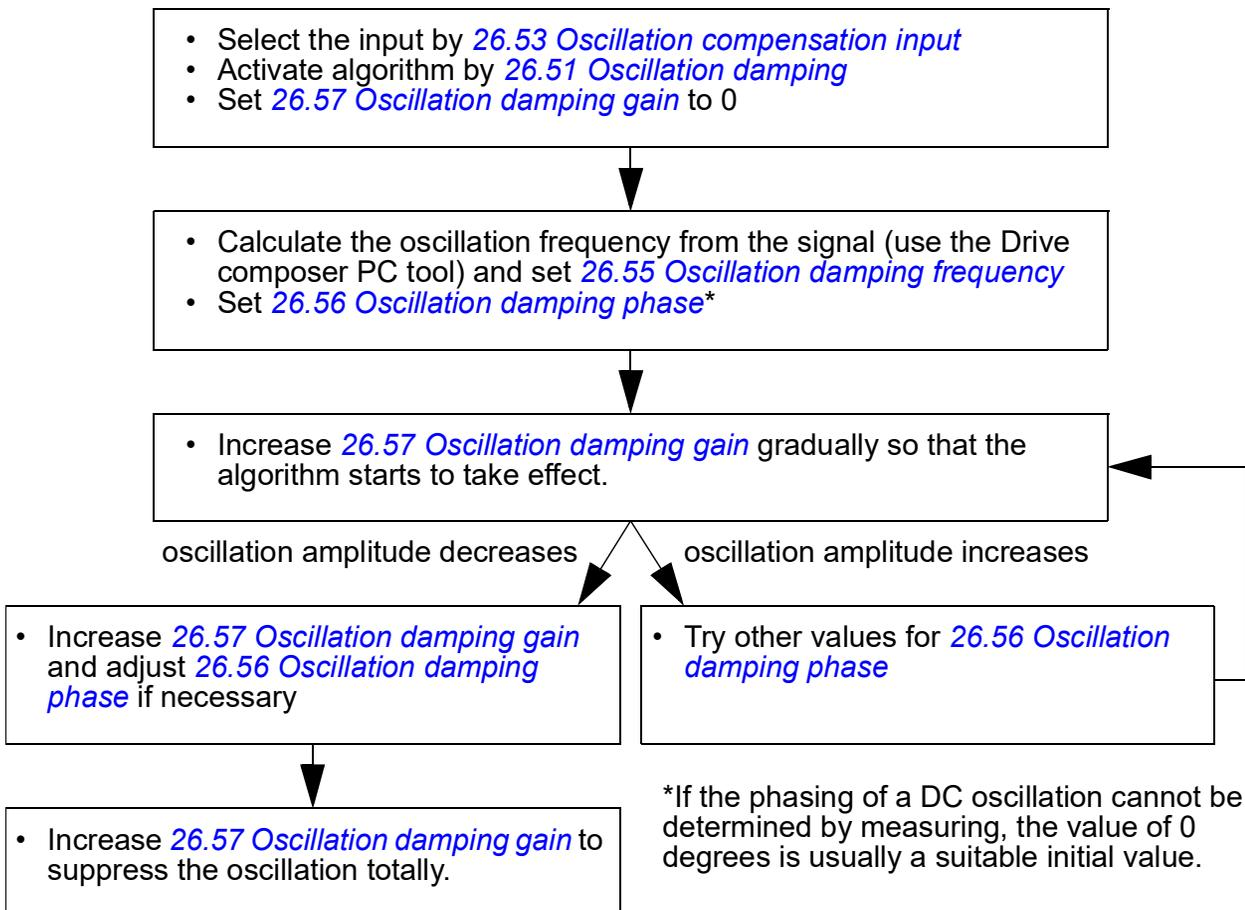
**Note:** Changing the speed error low-pass filter time constant or the integration time of the speed controller can affect the tuning of the oscillation damping algorithm. It is recommended to tune the speed controller before the oscillation damping algorithm. (The speed controller gain can be adjusted after the tuning of this algorithm.)
