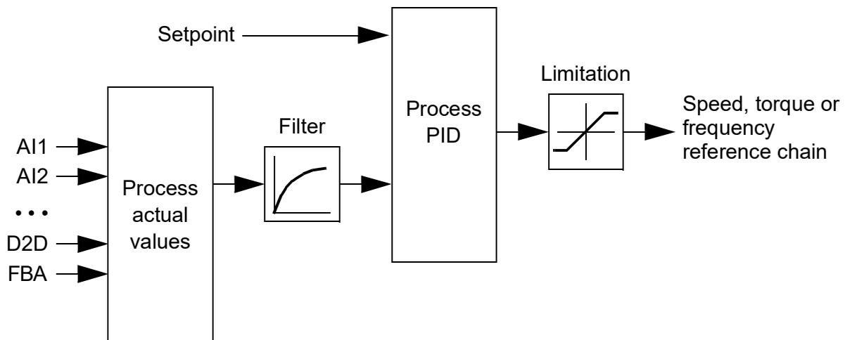
The control program contains two complete sets of process PID controller settings that can be alternated whenever necessary; see parameter [40.57 PID set1/set2 selection](#).
