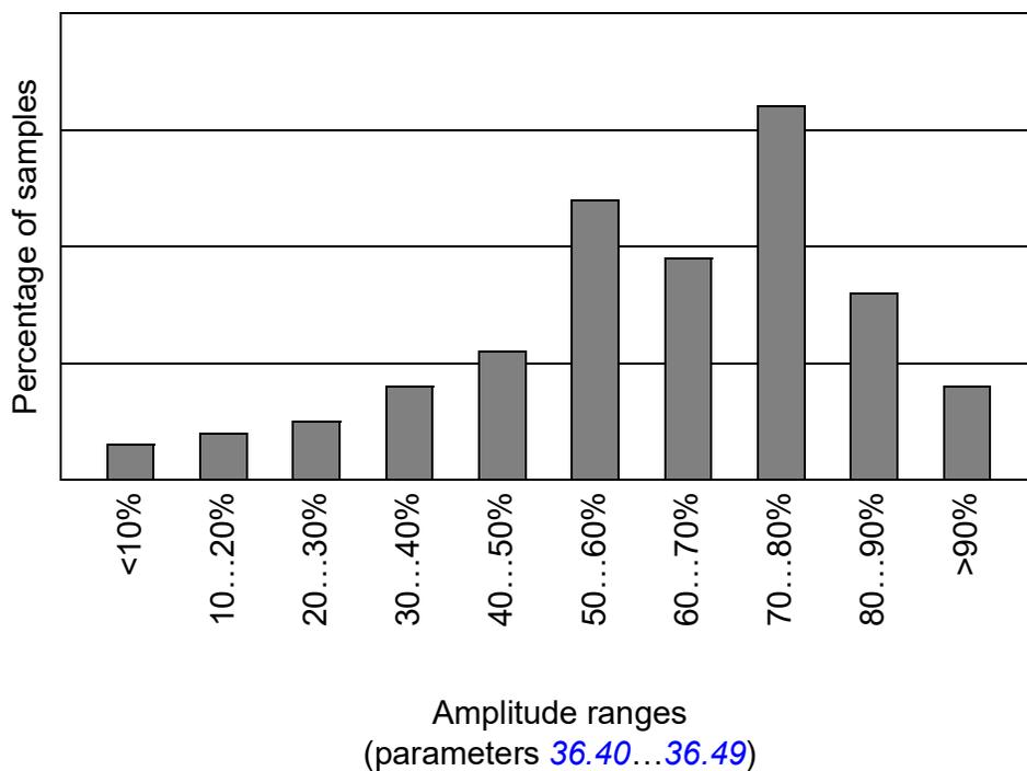
Amplitude logger 1 is fixed to monitor motor current, and cannot be reset. With amplitude logger 1, 100% corresponds to the maximum output current of the drive ( $I_{\max}$ , as given in the hardware manual). The distribution of collected samples is shown by parameters [36.20...36.29](#).
