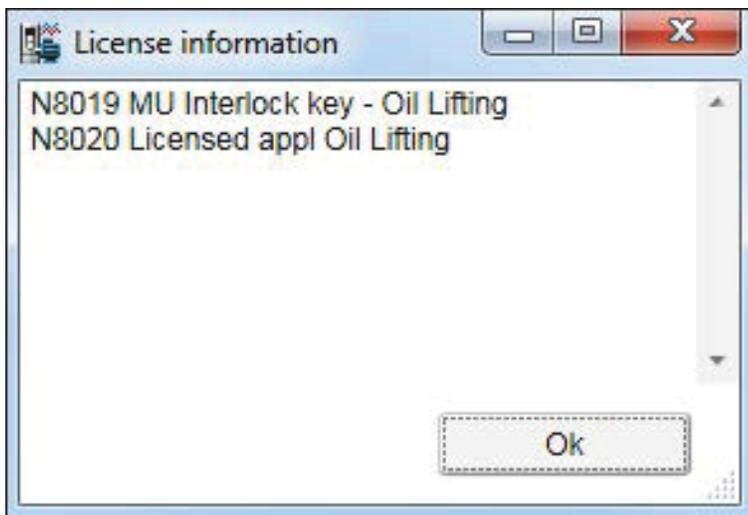
If the program was loaded to a ZMU-02 memory unit without the license key, then the drive indicates a fault [64A5 Licensing fault](#). See the auxiliary fault code in the Event logger to know the plus code of the missing license, in this case N8019. For further assistance, contact your local ABB representative.
