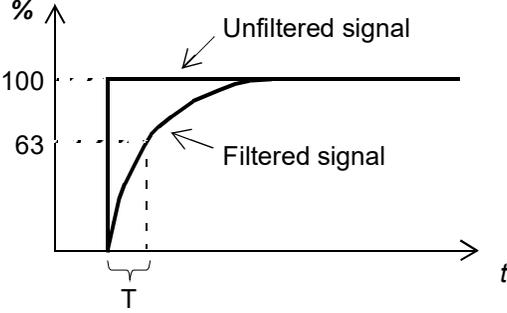
$O = I \times (1 - e^{-t/T})$ <p>I = filter input (step)<br/>O = filter output<br/>t = time<br/>T = filter time constant</p>                                                                                                                                                                                    | 0.0 s      |
