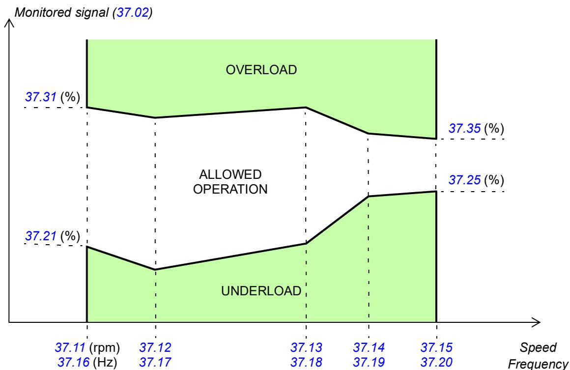
The action (none, warning or fault) taken when the signal exits the allowed operation area can be selected separately for overload and underload conditions (parameters [37.03](#) and [37.04](#) respectively). Each condition also has an optional timer to delay the selected action ([37.41](#) and [37.42](#)).
