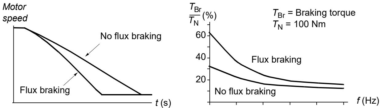
The drive monitors the motor status continuously, also during flux braking. Therefore, flux braking can be used both for stopping the motor and for changing the speed. The other benefits of flux braking are:
