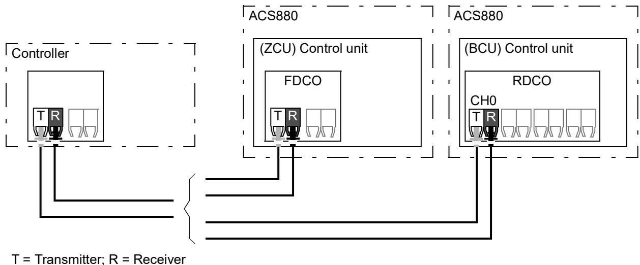
The external controller can also be wired to the D2D (RS-485) connector using shielded, twisted-pair cable. The selection of the connection is made by parameter [60.51 DDCS controller comm port](#).
