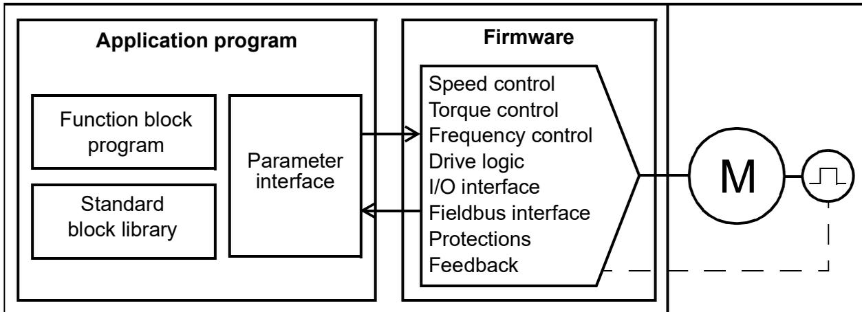
The firmware program performs the main control functions, including speed and torque control, drive logic (start/stop), I/O, feedback, communication and protection functions. Firmware functions are configured and programmed with parameters, and can be extended by application programming.
