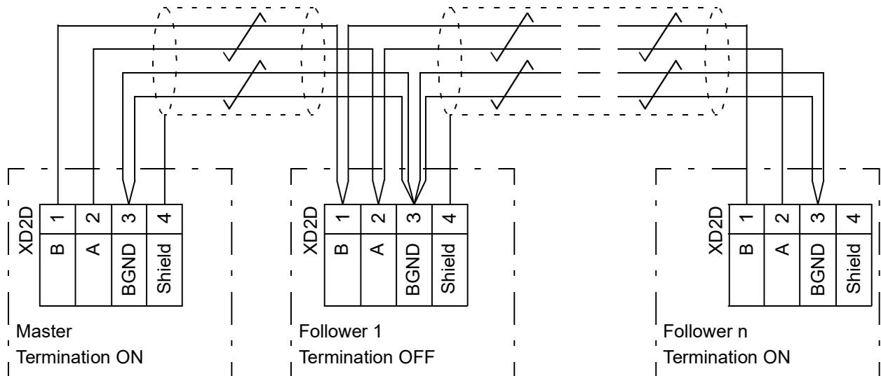
See the hardware manual of the drive for wiring and termination details.
