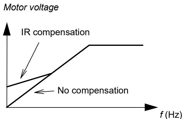
In Direct Torque Control (DTC), no IR compensation is possible or needed as it is applied automatically.
