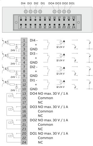
Figure 22: Electrical connections, digital I/O module
