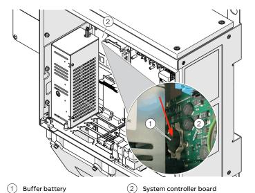
Figure 39: Buffer battery on the system controller
