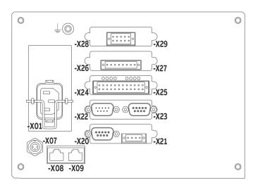
Image 16: Terminal assignment of electronic module (example)
