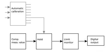
Figure 31: 'Limit value monitoring' application
