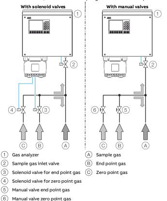
Figure 10: Sample gas discharge into the process
