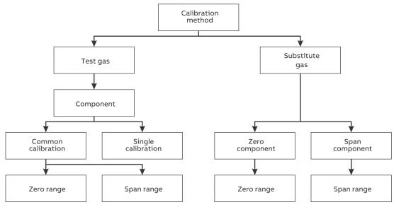
Figure 35: Adjusting the calibration method
