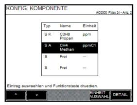
All the components of a detector are listed in this menu ('component list').
