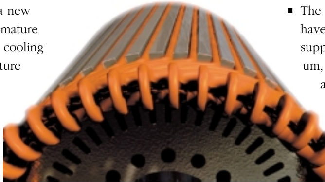
5 The armature coils are skewed for smoother running at low speeds and less noise.
