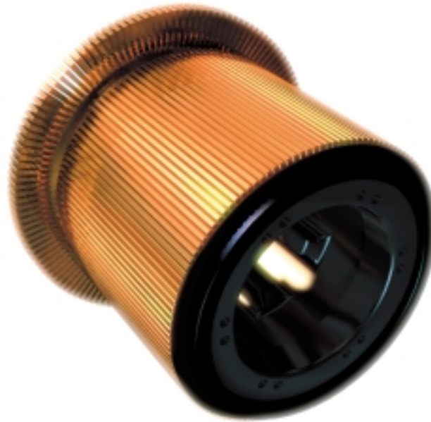
8 The commutator has a small diameter and therefore a low peripheral speed, ensuring that it will run properly even at high speeds.
