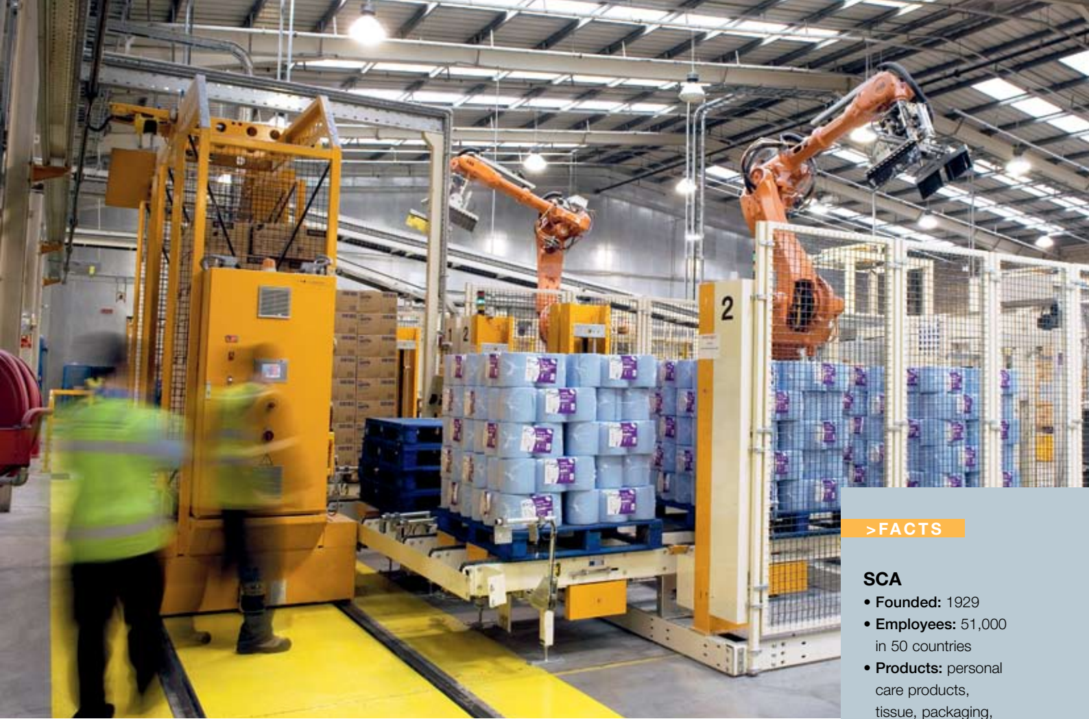
The IRB 6650 robots easily handle paper wrapped in shrunk polythene, a difficult material to work with.
