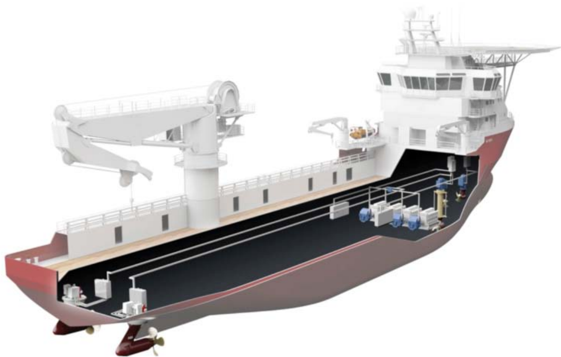
Simplified one-line presentation of the Onboard DC Grid. The main switchboards are removed from the configuration. Cabling is replaced by DC-bus.
