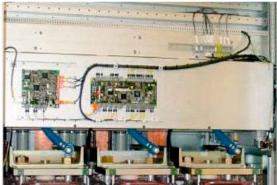
Module control cards are located in the segregated top section of the inverter cubicle. The control hardware is designed to be very simple. It also takes into account the Application Motor Controller card (not visible in the picture above).
