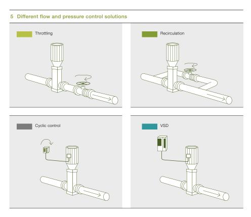
either a mechanical or an electrical solution. In many cases, pumps are operated at partial loads and thus enormous energy savings can be achieved by controlling the discharge pressure and flow by varying their speed rather than using throttle valves for mechanical control  $\rightarrow 4 \rightarrow 5$ .
