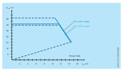
Hiccup mode, characteristic curve of output at  $T_a$  = 25 °C
