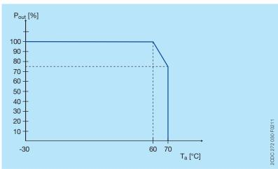
Characteristic curve of temperature at rated load
