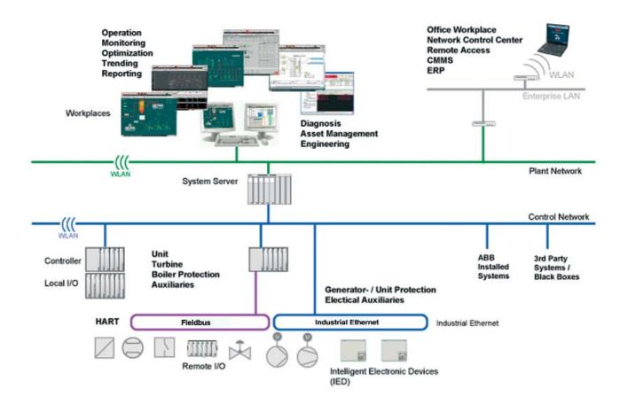
Fig. 1: Typical integration of DCS with instrumentation and electrical systems
