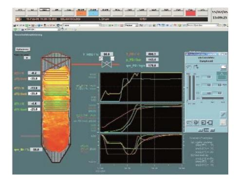
Fig. 5: Display of optimization results with OPTIMAX® BoilerMax
