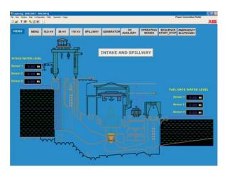
Fig. 3: Spillway control of a hydro power plant
