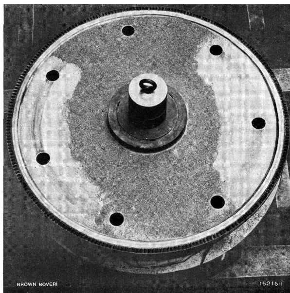
Fig. 3. — Vibration with one nodal diameter.
