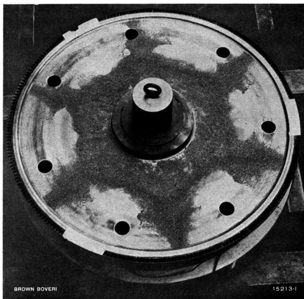
Fig. 5. — Vibration with three nodal diameters.
