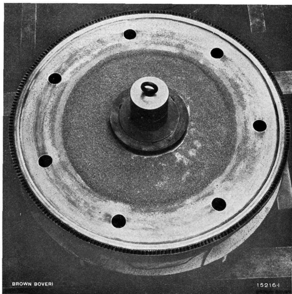
Fig. 2. Turbine disc with whole circumference vibrating without nodes.
