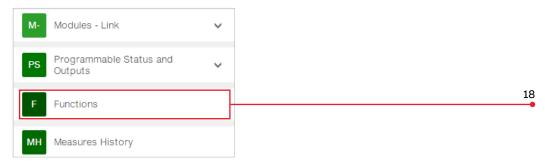
19. Under "Signalling Reset" click the "..." button for "Function". For "Trigger type" select "Custom." In the Trigger drop down, select "Ekip Signaling 2K input H." Change the X to 1 under Ekip Signaling 2k 3.2. Click "OK."
