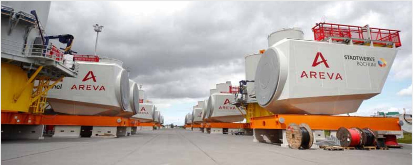
AREVA Wind M5000 nacelles in Bremerhaven ready to go offshore
