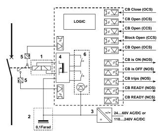
Figure 4: Block diagram of the control electronics
