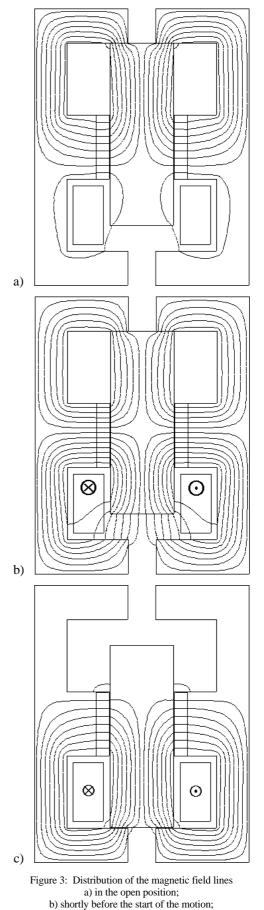
c) after the end of the motion and before switching off the coil-current
