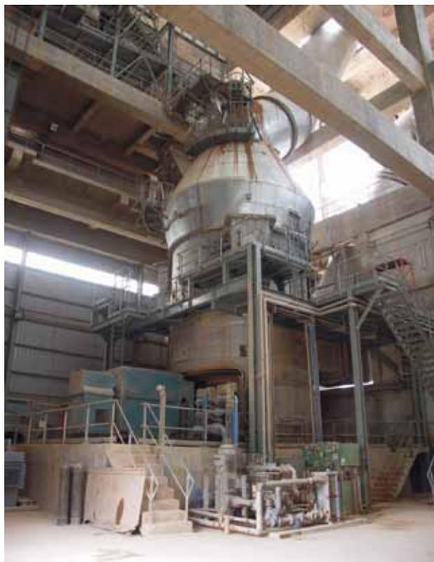
Raw mill with raw mill motor.
